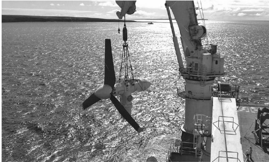
Mygen 18m 1.5 MW turbine in Pentland Firth, Scotland. Array by 2020 with output ~ 400 MW
